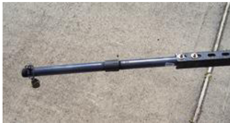
Figure 1: The PVC pipe and hoist pulley device mounted to the top of the Unistrut for hoisting the antenna.
