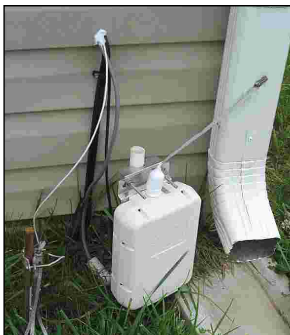
Gutter Set-up - The left photo shows the set-up of N8NQP's gutter antenna and the photo above is the back of his house with the gutter running the full length. The circle indicates the antenna coupler.
