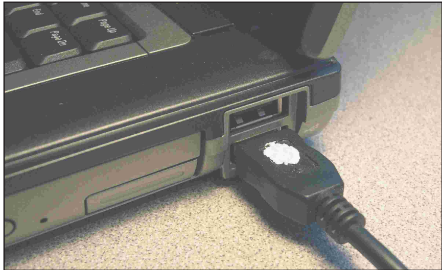
Place a drop "white-out" or white paint on the top side of cables to assist in the the orientation. (Photo by Tom Forrest, N4GVK)
