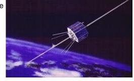
remained in operation until a short circuit occurred in a battery in 1981. More than 20 years later, however, AO-7 unexpectedly returned to life, its 2-meter beacon showing up on 145.9775 MHz. Satellite experts speculate that AO-7's resurrection occurred when the short circuit in the battery opened up for some reason, allowing the solar cells to power the spacecraft. When the satellite goes into eclipse, it powers down.
